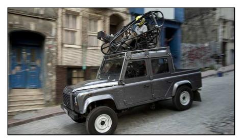
Most POD cars have been adapted purely for film purposes and so the vehicle no longer complies with construction and use legislation. The Road Traffic Act and construction and use regulations still apply to a public road, even one that is closed under a traffic order.
