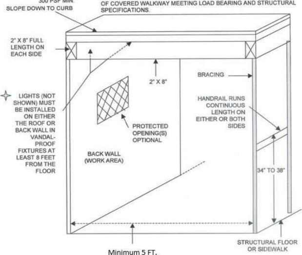
IF A STRUCTURAL FLOOR IS INSTALLED WALKWAY MUST INCLUDE
